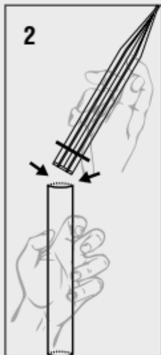
Turn stake upside down and insert firmly into extension tube.
