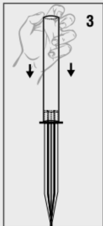
Attach ground stake's mounting bracket to extension tube and insert assembly firmly into the ground.
