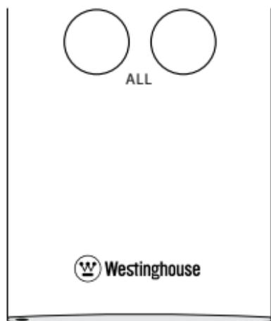
Using a phillips heads screw driver, remove the screw located at the base of the remote.
