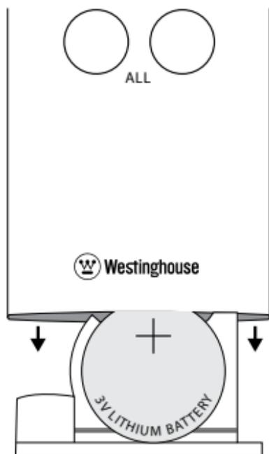
Remove the tray from the remote housing. Insert a new CR2032 lithium battery into the battery holder. Make sure to correctly position the + (positive side of the battery) face up. Push the tray back into the remote housing and secure it in place with the screw.
